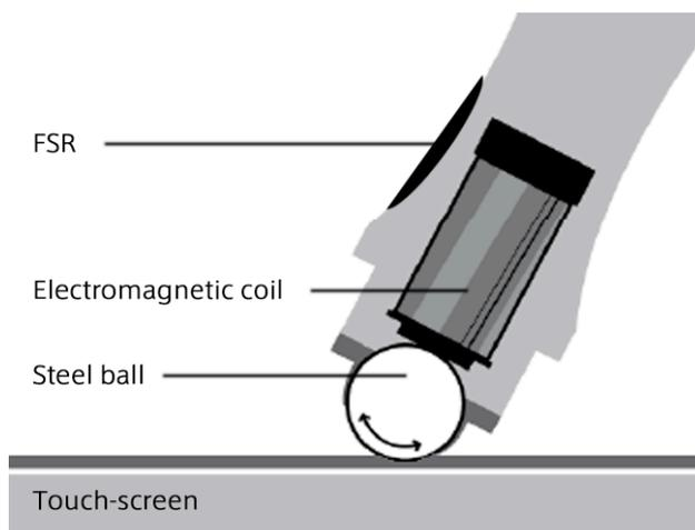
Figure 1. Setup of screen, stylus and FSR
